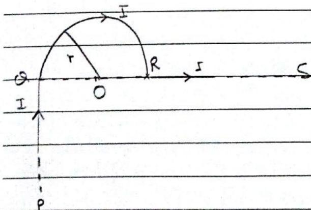
$$B_{\text{due to PQ}} = \frac{\mu_0 I}{4\pi r} (\sin 90^\circ + \sin 90^\circ) \\ = \frac{\mu_0 I}{4\pi r} \cdot 2 = \frac{\mu_0 I}{2\pi r}$$
