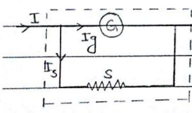
let G be the resistance of the galvanometer and s that of the shunt. I<sub>g</sub> is the current through the Galvanometer and I<sub>s</sub> be the current through the shunt then  $I = I_g + I_s$
