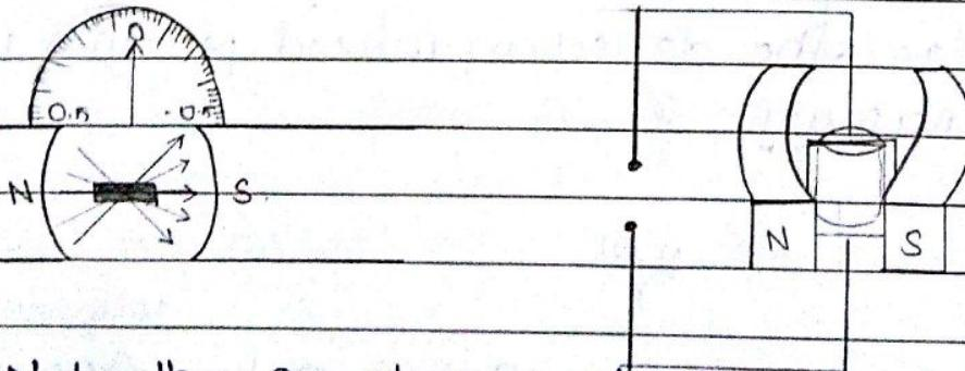
Let  $N$  be the no. of turns of the coil, and  $A$  be the area of cross section. The ends of the coil are connected to a source of voltage. When the circuit is switched on the loop will experience a torque and is given by
