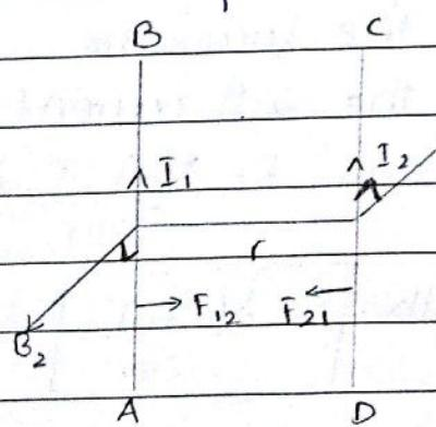
Magnetic field on CD due to the current  $I_1$ ,
