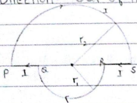
$$B \text{ due to PS} \quad B_1 = \frac{\mu_0 I}{4r_2}$$
