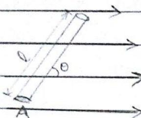
let  $n$  be the no. of free electrons per unit volume and  $V_d$  be the drift velocity.
