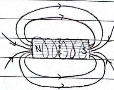
The polarity of solenoid is determined by the direction of current. If the current at one end of the solenoid is flowing in clockwise direction, that end is the south pole and if the current is flowing in anticlockwise direction that end is the north pole.
